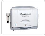
Air Generators produce dry and hydrocarbon-free air (NOx/SOx free and CO<sub>2</sub> free with GT series) by using air from oil free compressors, thus avoid the need to use conventional bottles that are often complex to change. With this zero air, you can decrease the background noise level because it gives the baseline much better stability, considerably increasing detector sensitivity and ensuring precise analytical results.
