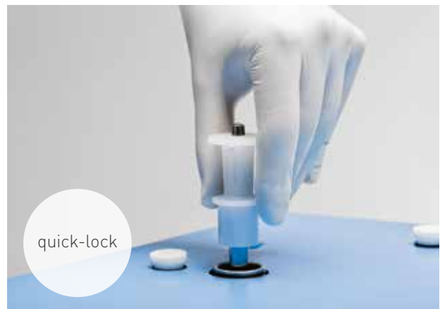
→ Fixed shaft height with quick-lock system
